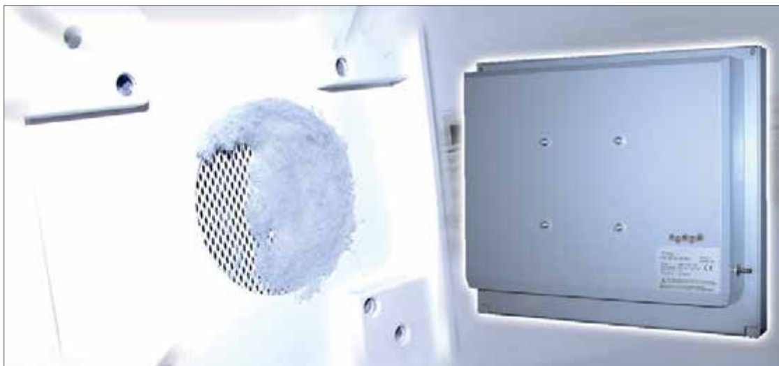
Figure 3: Dust and particles from the ambient air often collect on ventilation slots.
